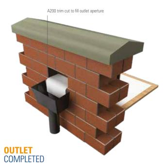
To allow water to flow into the gutter an 'A' type drip trim should be used. In order to allow the drip trims to sit level with the roof and to prevent water from ponding in the outlet, the board forming the outlet should be rebated by 3mm.
