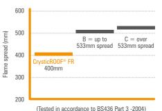
CrysticROOF® FR is specifically designed to meet British fire standards. The CrysticROOF® FR system includes an FR resin and FR topcoat that combine to meet British fire standard BS 476: Part 3.
